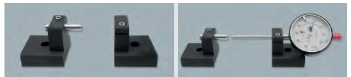
Controllo comparatori / Control de comparadores
